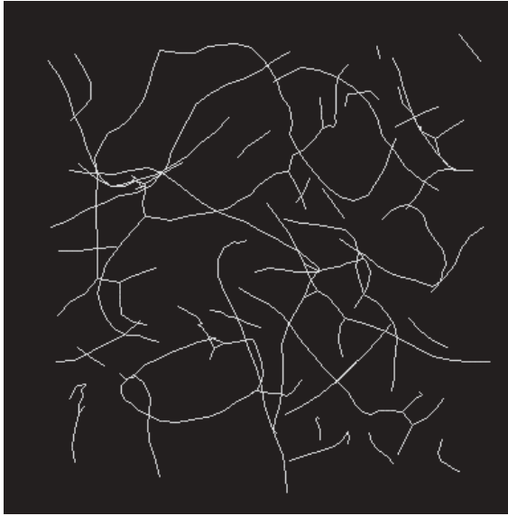
Fig. 5.14. Sample snapshot of a realization of a system made of FENE-CB6 chains (5.32). Beside scissions/recombinations of chains (parameterized through a scission energy E_{sc} ) the model allows for the formation of branchings and carries a parameter for the (in plane) stiffness of chains. The concentration is c = 5\% . Results obtained via BD
